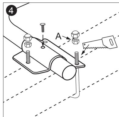
The height of the frame of the drawbar determines the cutting of the thread.
